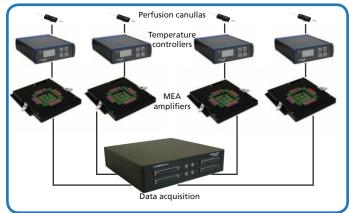
MEA amplifiers are available in two different versions, designed specifically for upright and inverted microscopes.
