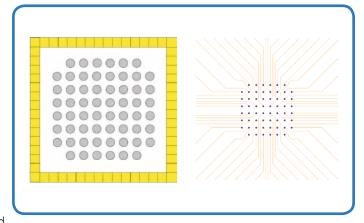
low noise level. 10 µm electrodes enable recording from single neurons or single cardiomyocytes.
