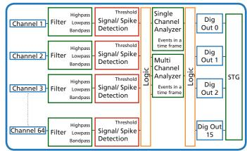
analysis, and feedback logic happens on a special signal processor unit within the USB data acquisition. This bypasses the PC altogether to speed up the process. With real-time signal detection and feedback, it is possible to enable communication between devices accepting TTL pulses as a trigger without delay.
