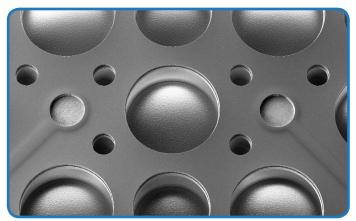
acute slices. In addition, slices can be held in stable contact with the MEA surface by applying a negative pressure, thereby sucking the tissue down to the electrodes. A slice anchor (weight) is no longer necessary.
