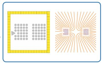
The main application of this MEA type is high resolution recording of individual neurons in neuronal networks. The electrode diameter is 10  $\mu m.$  A low noise level is guaranteed by the use of TiN as electrode material.
