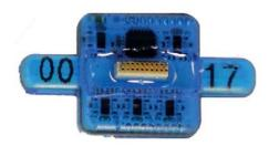
W8-Headstage bottom side: Connector for the electrode probe or the ME/W-Signal generator via the adapter ADPT-Om-ME/W-SG.
