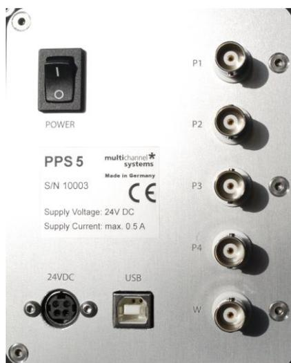
1. Connect the provided power supply to the "24VDC" connector.
