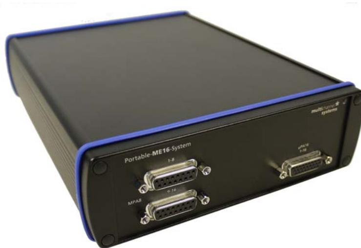
The Portable ME16-System can be used either with two MPA8Is - or - with one  $\mu$ PA16. The device is preconfigured by Multi Channel Systems and cannot be modified by the user. If you like to change the preconfiguration, please contact MCS: [www.multichannelsystems.com](http://www.multichannelsystems.com)
