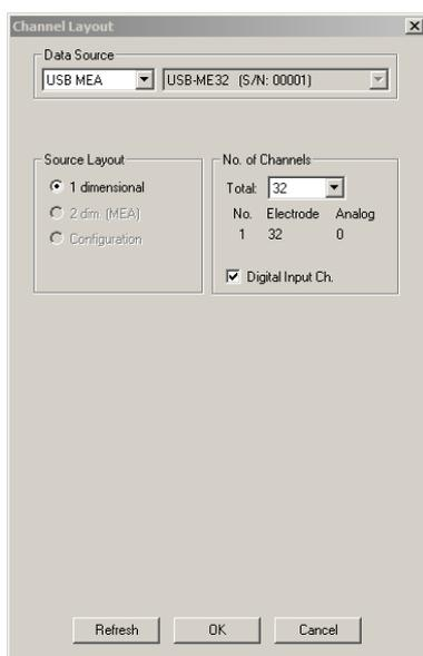
MC\_Rack now recognizes the Portable-ME System as data source. For further instructions how to use the MC\_Rack software please refer to the respective manual and help files available on the web site and as online help in MC\_Rack.
