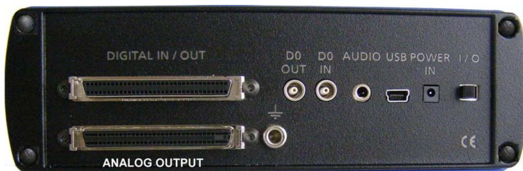
Analog signals are splitted between the filter amplifier and the A / D converter. The additional analog output on the rear panel of the Portable ME-System has the same pin layout as the output of a FA32 (32-channel filter amplifier). Please see pin layout below.
