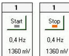
The option "**Start**" for channel 1 appears when no waves are downloaded. The option "**Stop**" for channel 1 appears when program is running.
