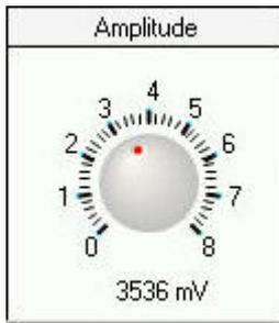
Select the amplitude of the pulse. The unit is millivolt (mV). Click onto the red point of the control dial and move it while keeping the left mouse button pressed. The exact value of the amplitude will be displayed below the control dial.
