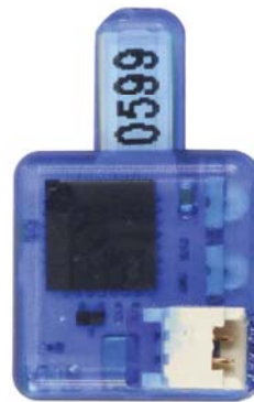
W4-Headstage top side: The white connector is for the storage battery. Please use this connector for orientation of the headstage.
