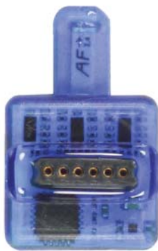
W4-Headstage bottom side: Connector for the electrode probe or for the ME/W-Signal generator
