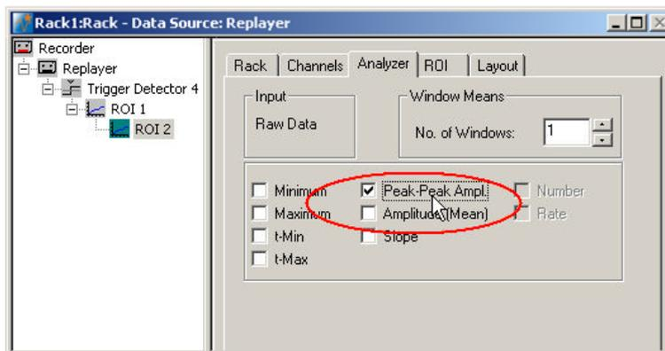
5. Click the **ROI** tabbed page. The recording trigger **Trigger 1** is already preselected, but you can also select the **Trigger 4** that is generated by the **Trigger Detector 4**.
