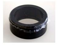
In order to allow long term cultivation and recording, Multi Channel Systems MCS GmbH recommends the use of teflon membranes (fluorinated ethylene-propylene, 12.5 microns thick) developed by Potter and DeMarse (2001). The ALA-MEA-MEM membrane is produced in license by ALA Scientific Instruments Inc., and distributed via the world-wide network of MCS distributors.
