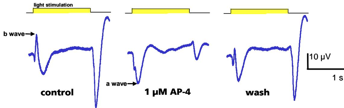
Drug action on a light-evoked microERG. Application of the glutamate analog AP4, a blocker of the on-signal pathway in the retina, resulted in the separation of the a-wave by elimination of the b-wave. The b-wave amplitude is restored after drug wash out.
