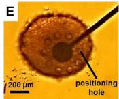
View of a Beta-Screen electrode covered with an intact murine islet positioned via negative pressure through the positioning holes.
