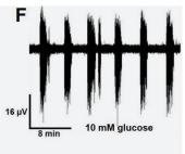
Typical field potential recording of a murine islet with characteristic oscillatory activity in 10 mM glucose.
