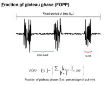
The fraction of plateau phase (FOPP) is the percentage of burst activity in a time interval. FOPP is a marker for insulin release.
