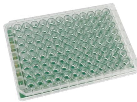
The 96-well plates feature 3 electrodes per well. In all well plates, there is an internal reference electrode in each well and each electrode can be selected for stimulation.
