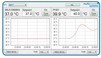
The screenshot on the left shows the stability of the temperature controller on channel 1 and the quick reaction on a setpoint temperature change on channel 2.
