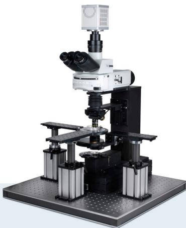
uM-Scope for dual patch clamp and wide field fluorescence imaging: XYZ-motorized microscope, transmitted light illumination, dual uMp-3 manipulator system and rigid posts for the manipulator and sample mounting:
