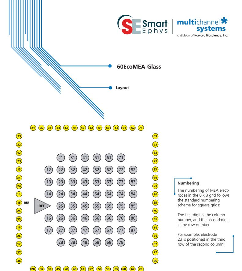
The MEA Electrode IDs are the channel numbers that are used in the data acquisition program. When using MC\_Rack software, please select the 2 dimensional layout (or Configuration) in the "Data Source Setup". Electrode 15 is missing in this MEAs. It is replaced by a big internal reference electrode, connected to pin 15 of the amplifier.
