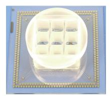
The 9well-CC mounted together with a 9well macrolon quadrat on a 256-9wellMEA300/30iR-ITO.
