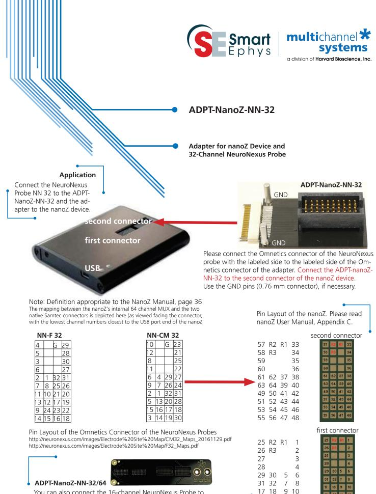
You can also connect the 16-channel NeuroNexus Probe to the ADPT-nanoZ-NN-16, and then via ADPT-nanoZ-NN-32/64 to the nanoZ device. The ADPT-nanoZ-NN-32/64 is available from Multi Channel Systems and has to be ordered separately.
