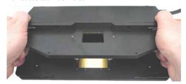
The longer screws (M3x12) belong to the bore holes on the right and left periphery of the contact unit. The shorter screws (M3x10) belong to the bore holes in the centre of the contact unit beside the open area for the MEA chip.
