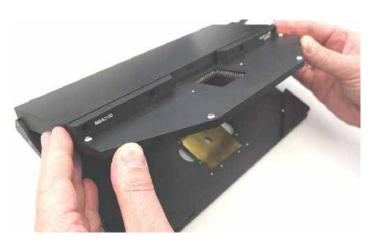
3. Place the new contact unit in front of the MEA2100 device. There are guide bars on the left and on the right which help to reconnect the contact unit. Connect the connector pins of the contact unit to the connector sockets of the MEA2100 headstage. Push the new contact unit carefully for reconnecting. Use the provided screws to fix the contact unit.
