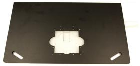
Turn the ground plate of the MEA2100 headstage around and put it onto a soft surface to avoid scratches. You need a TORX T6 screw driver to remove the designated screws (M2 x 4). Unscrew the six screws which fix the cover for the tubing. Keep the screws for reusing them later.
