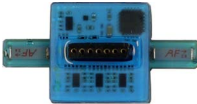
W2100-HS-EEG/EMG/Temp bottom side: Connector for the electrode probe or the ME/W-Signal generator.
