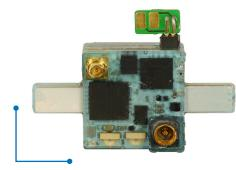
The adapter for external stimulation has to be connected magnet to magnet to the headstage. Please solder a connection wire to the pads provided on the adapter.
