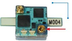
**W2100-HS8-ES2-EXT** top side Please use the connector for the storage battery in the lower right for orientation of the headstage.
