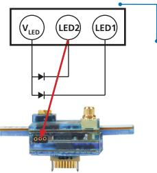
**Connector for optical Stimulation** An additional connector with three pins is available for the optical stimulation via LED: Connector from Mill-Max 1 mm Pitch: 861-13-050-10-002000 + Magnet-cuboid Magna QA-3x1x1-N45-N on the headstage mates with Mill-Max 1 mm Pitch: 860-10-050-10-002000 + Magnet-cuboid Maqna QA-3x1x1-N45-N)
