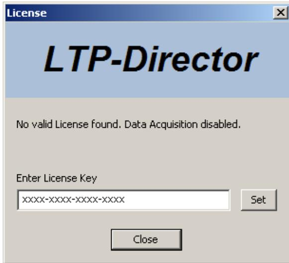
The LTP-Director software license is bound to one dedicated hardware device. The license key will be saved on the device. The license key does not unlock the software – as usual – but the hardware. This way it is possible to connect the device to different data acquisition computers.
