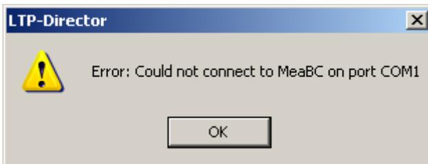
If you start the LTP-Director in Test Mode, the software tries to connect the MEA1060 amplifier. Please select the correct COM port from the drop down menu "MEA-BC Port" in the Control Window for connecting the MEA amplifier.
