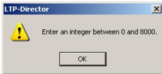
The amplitude of the stimulus test pulse has to be an integral number in a range between 0 and 8000 mV. Please select an appropriate value.
