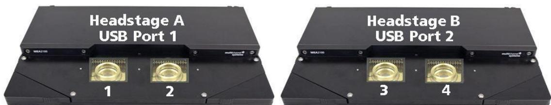
Click "Hardware" tab in main menu "Settings" in the first instance of LTP-Director and select the MEA2100. You can adjust the input voltage range and the sampling frequency for both connected headstages and each of the 60-electrodes MEA.
