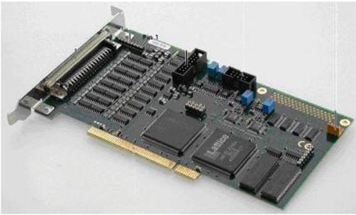
The **MC\_Card** is the data acquisition card of MEA- and ME-Systems from Multi Channel Systems MCS GmbH. Please see also the separate documentation of the systems and its components for more information about the setup and operation.
