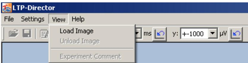
It is possible to load a photo as background picture into the electrode field of the "Test Mode Control Window". You have the direct optical control of the position of your stimulation and recording electrodes.
