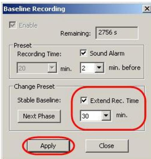
To extend this phase, click the "**Extend Recording Time**" marker. Now it is possible to increase the duration of that phase while experiment is running.
