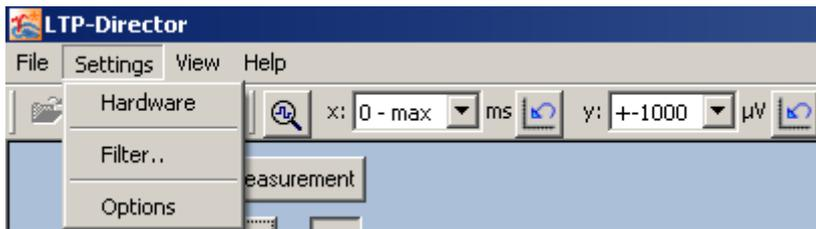
In the settings menu, the hardware configuration, the filter parameters, and several options can be defined. To define the hardware settings, click the "**Hardware**" tab under "Settings".
