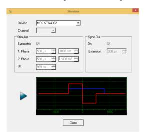
You can connect either one stimulus generator STG with more than one channels, or several STGs to stimulate the different ME amplifiers. Define either the channel number from the "Channel" drop down menu when using one STG, or the devices from the "Device" drop down menu when using several STGs.
