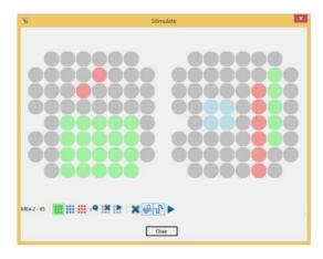
The dialog mirrors the layout of the currently used MEAs, in this case a MEA2100-2x60-System with two slots for two 60-electrode MEAs. Use the tool bar thereunder to define the stimulation sites.
