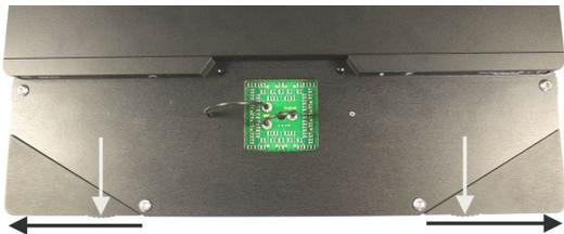
The two triangular front edges of the device can be moved outwards and inwards to open and close the MEA-IT device, respectively.
