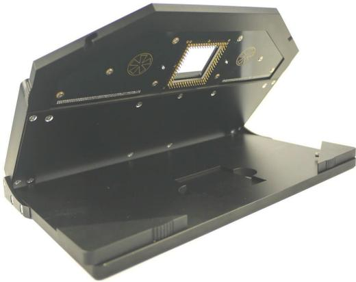
The MEA-IT is a very compact and portable device for measuring electrode impedances on microelectrode arrays (MEA) with MEA-IT software.
