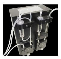
Peristaltic perfusion system PPS2 with one inlet and one outlet pump. Both pumps can be operated independently, or inflow and outflow can be linked, the percentage difference is adjustable. For setting up the pump, please read the "PPS2 Manual".
