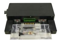
Connect the complete MEA chamber to the MEA2100-Beta-Screen headstage. Insert the tubes carefully into the respective slots and connect the adapter to the provided plug in.
