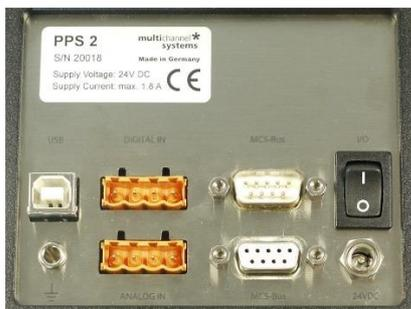
1. Connect the PPS2 pump with the provided power supply cable to the power supply.
