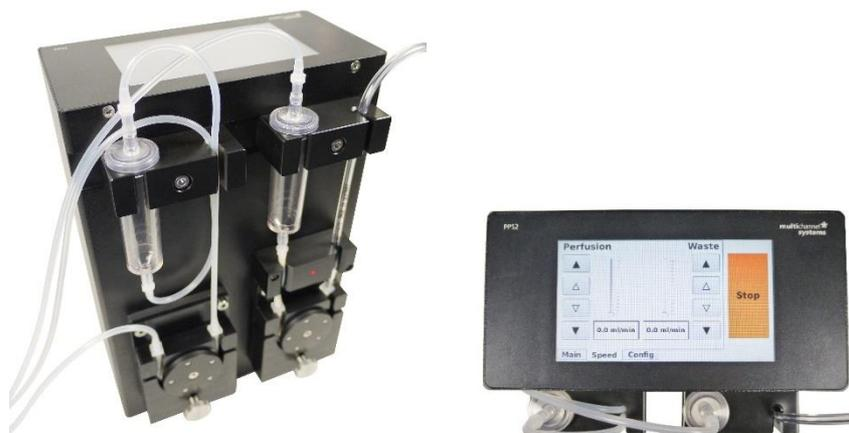
The **peristaltic pump PPS2** with **software control** is developed for the perfusion of biological samples. The pumps are driven by stepper motors providing a very long lifetime without maintenance. The durable brushless motors are extremely reliable, show very constant rotation speed, are vibration free and have low electromagnetic emission. These characteristics make the PPS2-System an ideal choice for electrophysiological experiments.
