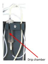
The drip chamber (droplet isolator) can be used to disrupt the direct liquid column from the pump to the sample. This can help to remove low frequency noise originating from the pulsation of the pump head. On the other hand, the droplet isolators make the flow speed inaccurate, and cause a continued flow even after the pump is stopped. If the flow rate is high (approximate > 6-8 ml/min) the droplet isolators will fill up over time and might even overflow.
