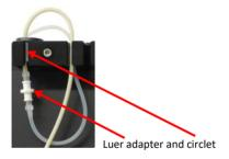
If you do not need the drip chamber, please use the circlet and connect the heads of the tube with a luer adapter.
