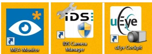
Use the **IDS Camera Manager** software to execute the camera. The **uEye Cockpit** software is an universal visualization software and **MEA Monitor** a visualization software, optimized for the MEA video microscope tables from Multi Channel Systems MCS GmbH. It is mandatory to install the uEye software before installing MEA Monitor.
