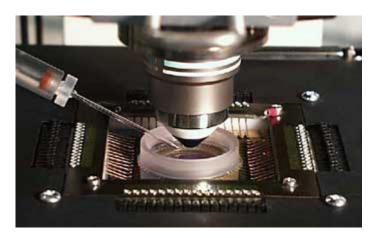
Raw data from up to **60 electrodes** of a **microelectrode array** (**MEA**) is amplified by **60 channels** of **filter amplifiers** that are built very small and compact using SMD (Surface Mounted Devices) technology. The small-sized MEA amplifier combines the **interface** to the **MEA probe** with the **signal filtering** and the **amplification** of the signal. The compact design reduces line pick up and keeps the noise level down.
