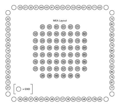
The illustration shows the standard pin layout of the socket on the amplifier. The list below shows the assignment of the electrodes to the pins of the socket. Pin 1 is the ground of the power supply, pin 2 is the ground of the signal, that is, where the signal is referred to. Both pins are already internally connected inside the amplifier.
