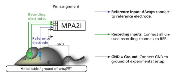
Important: It is important that the **complete setup** refers to a **single common ground**. The **reference input** has always to be connected. It is recommended to use a **reference electrode**. However, if you are not using a reference electrode, connect the reference input to ground (GND). Otherwise, noise picked up by the reference input will be subtracted from the recording signals. This will either lead to signal loss or to a very high noise level.
