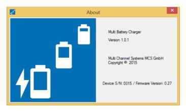
The "About" dialog shows the version number of the actual Multi Battery Charger software and firmware version. Additionally the serial number of the Multi Battery Charger device is displayed.
