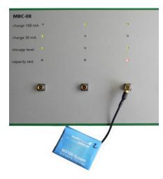
The red LED for the capacity test is flashing slowly during the test is running and off after finishing the test.
