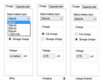
Please select the type of the battery before the battery is connected. Select in the "Charge" window the mode "Full charge" or "Storage charge" via radio button. In the "Voltage" window the state is displayed. In the footer below the actual working phase is indicated, for example "idling" if no battery is connected, "charging" or "discharging" together with blue status bars, when working.
