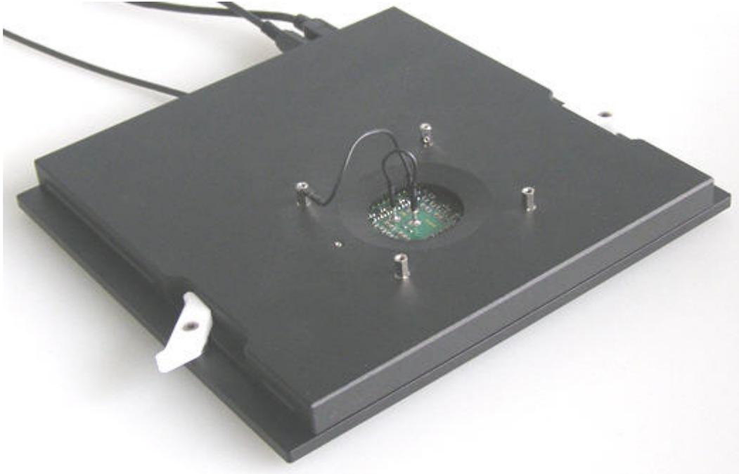
The USB-MEA1060 is a very compact and portable stand-alone solution. It features an integrated 60-channel filter amplifier and data acquisition. The digitally converted electrode signals are transmitted to the connected computer via universal serial bus (High Speed USB 2.0). Thus, it is possible to use any computer as a data acquisition computer, also a laptop. The size of the complete system is small enough to fit into a laptop bag together with the computer.
