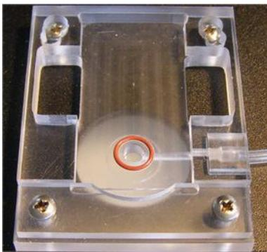
Place the Test-MEA32S12-Lx **test model probe** inside. Replace the upper unit, and close the holding clamps carefully.
